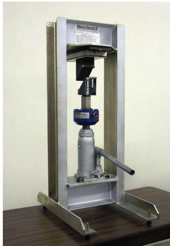
Model 810 shown here mounted in an optional testing frame with a load cell.
