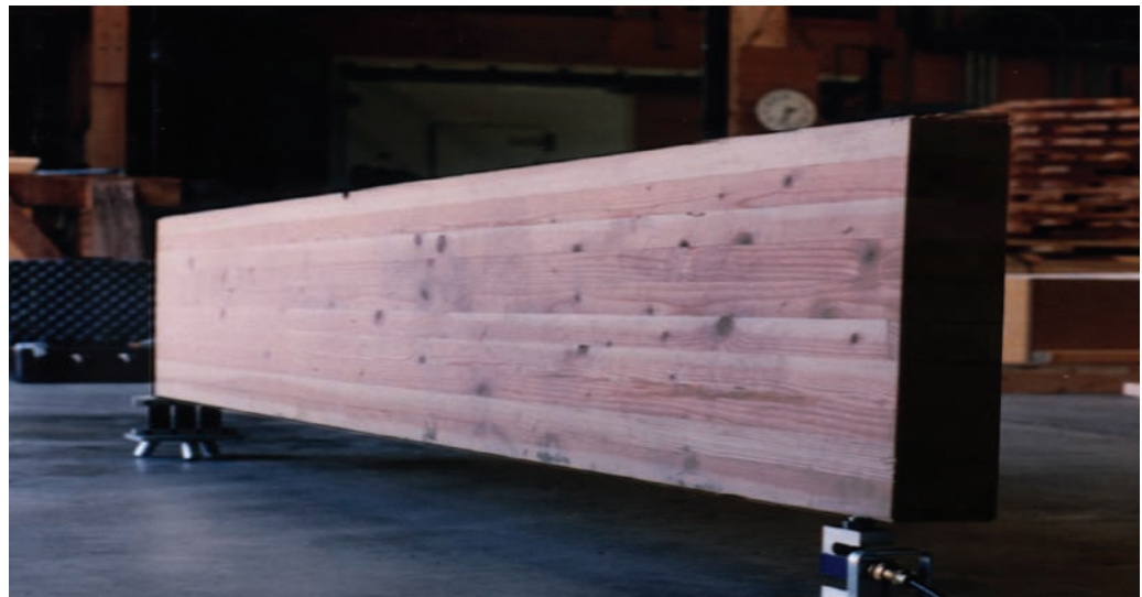
A laminated beam, ready for testing, rests on the tripod test fixtures without the tripod legs attached.
