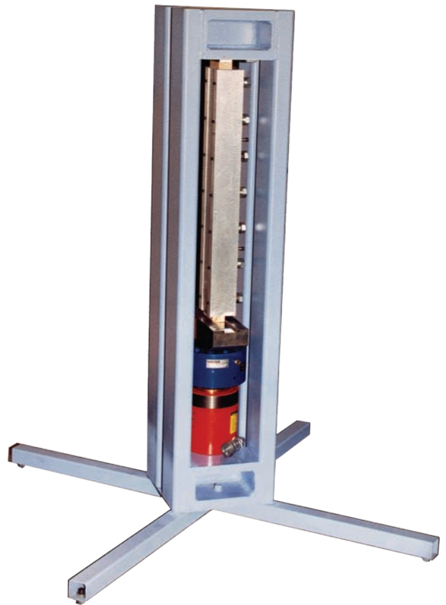
Model 870 Compression Parallel Tester with a 2x4 specimen mounted in the testing frame.
