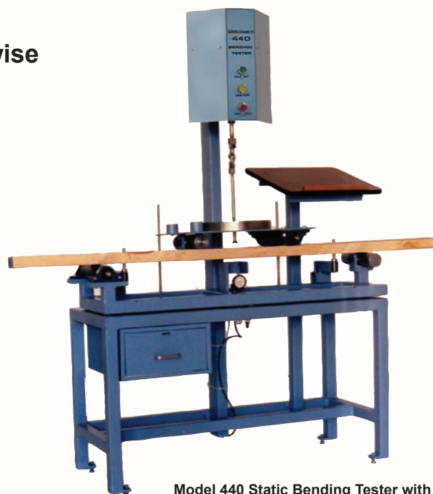
Model 440 Static Bending Tester with test specimen ready for loading.
