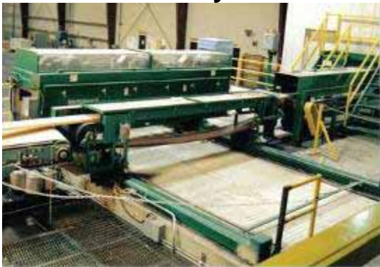
Shifting Base & Bypass Conveyor
