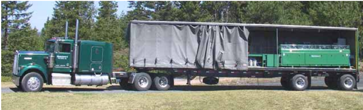
Figure 5. Metriguard's mobile MSR system can provide an on-site evaluation of your MSR yield potential. This is a self-contained system with its own diesel engine driven 3-phase generator set, and it can be up and running in a few minutes after arriving at your mill site. We can provide this service at a reasonable charge to cover our costs for fuel and labor.
